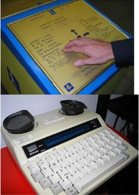
The top photograph shows a person's hand touching a Braille display on a blue frame. The bottom photograph shows a white Braille keyboard with a small screen and a Braille display on top. |                                                                                                                                                               |  |
